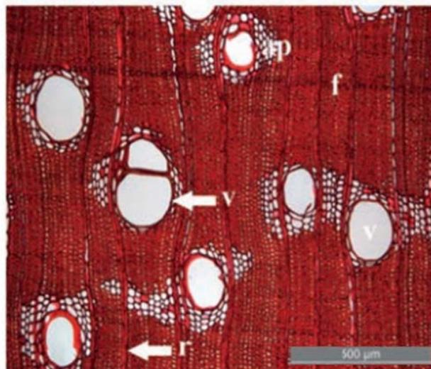
**Figure 4** Cross-section of *A. cucullata* wood showing very low vessel density (ap = axial parenchyma, f = fibre, v = vessel and r = ray) (From Khaopakro *et al.*, 2015).
